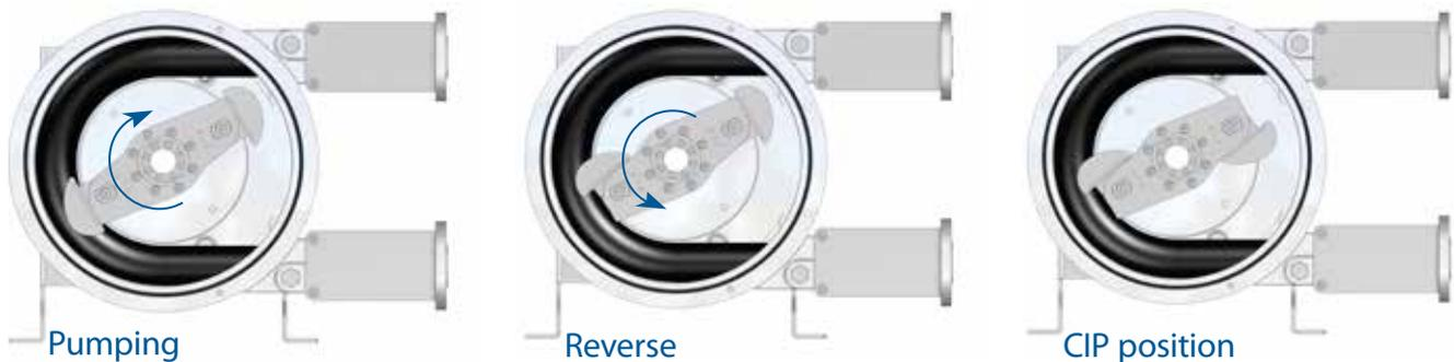
PT pumps are available in "CIP wheel" (Clean In Place) option. It allows users, by simply reversing the direction of rotation of the pump (1/2 turn), to be able to retract the shoes automatically, in order to make the cleaning and sterilization operations, without any action on the pump. The client saves time and will keep the highest level of functionality in the process.
