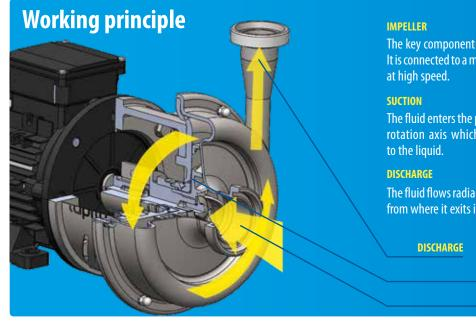
The key component of a centrifugal pump is an impeller. It is connected to a motor through a drive shaft and rotated at high speed.
